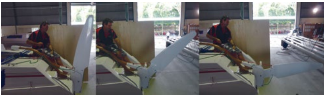
Cruze 970 transom hung rudder being lifted up
