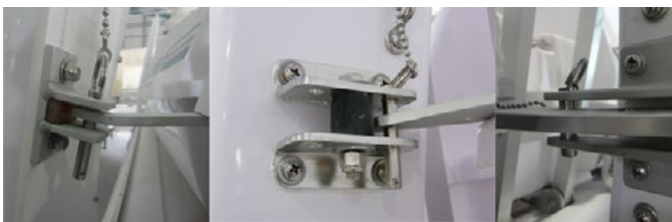
Beam locking pin: 750/C28/Cruze 970
