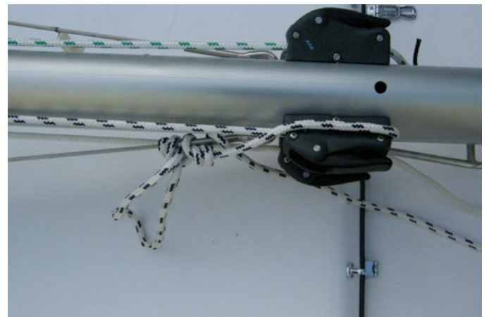
Halyard tied down as safety back up
